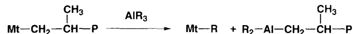
Scheme 1 Chain transfer reaction in propylene polymerization: Mt = metal, and P = polymer chain.
